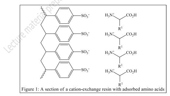
The strength of the adsorption varies with the basicity of the individual amino acids. The most basic amino acids are held most strongly. The column is then washed with a buffered solution at a given pH, under this condition the individual amino acids move down the column at different rates and ultimately become separated. The rate at which each amino acid emerges from the column under very carefully defined conditions is accurately known from the standards.
